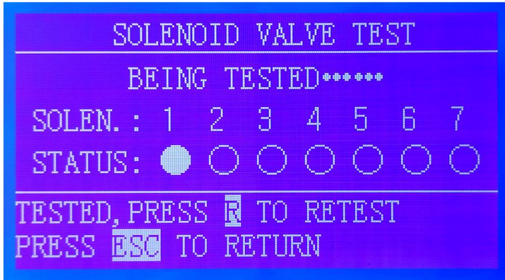
Under the solenoid valve test menu, the machine will automatically test each solenoid valve; when the test is finished, press the “R” key to re-test the test, press the “Esc” key to stop the test and return to the previous menu.
