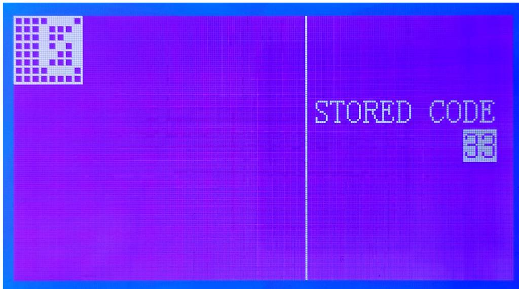
Press the number keys to enter the graphic code to be modified, and the corresponding graphic will be automatically called up for the user to edit. After the modification is completed, press the Enter key to save the graphic. Viewing Graphical Information Viewing graphical information allows the user to easily view stored graphical information.
