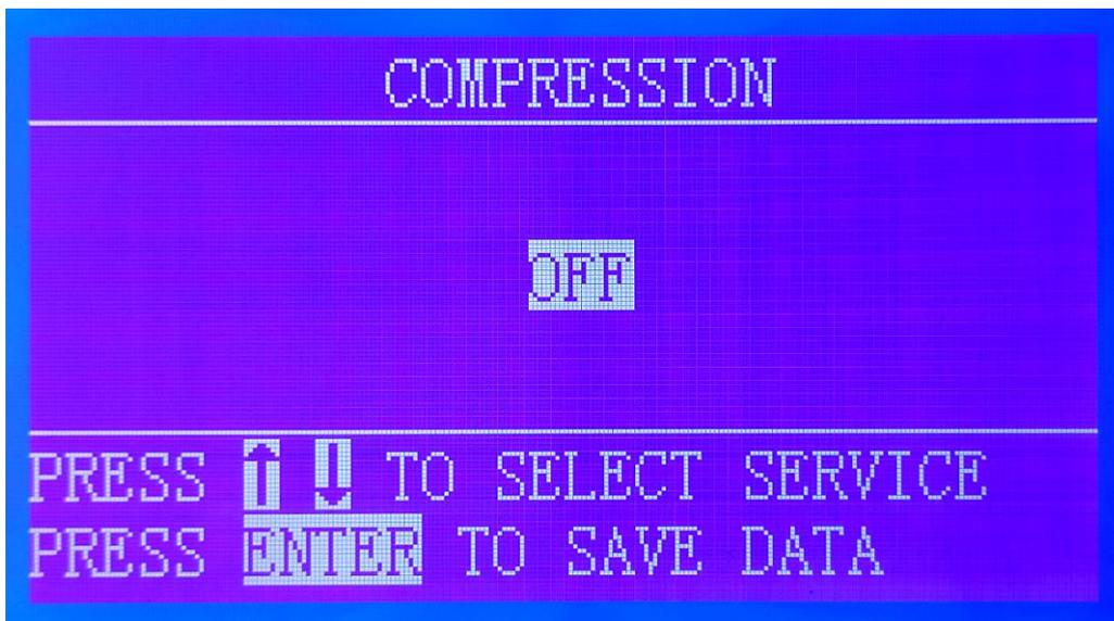
Under the compression settings menu, use the “↑ ↓” to select the compressed value, and the system defaults to compression off state, adjustment range: close 7,6,5. After the setting is complete, press “Enter” to save the data and return to the previous menu. If you need to return to the previous menu without saving the data, press “Esc” directly.
