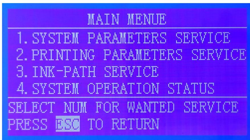
Under the main setting menu, press the number key to enter the corresponding setting menu, and press Esc to return to the previous menu.
