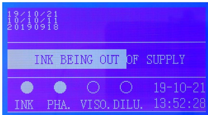
After the stop ink supply process, the screen returns to the boot default display state.
